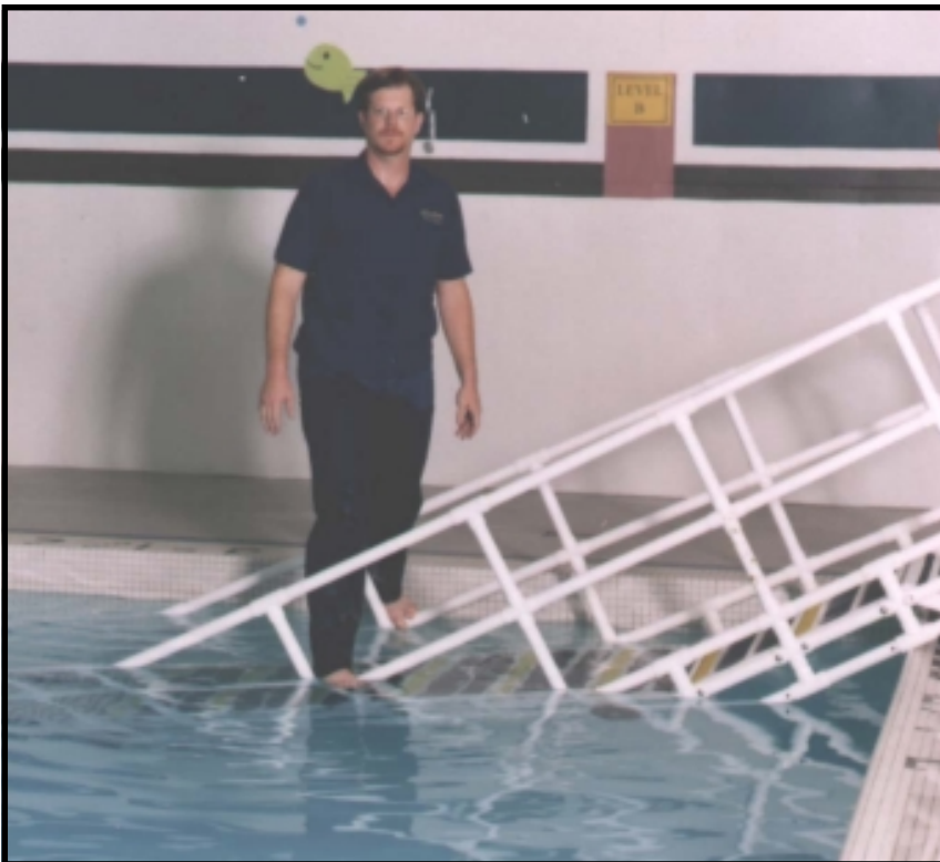
Above: Perry Sawrey, Managing Director, stands on top of the siderails of an AQ-9000 AquaTrek Ramp to demonstrate the durability and strength in the siderails. As you can see, this 6’5” 285 pound man is easily supported by the rails.
